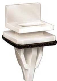
17096 (91513-SM4-000) Nylon Rocker Panel Moulding Clip Width: 20mm Length: 20mm Fits into 12mm Hole Accord 1991 - On
