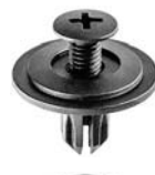
14698 (90688-SB0-003) Black Nylon Push-Type Retainer Head Diameter: 18mm Stem Length: 11mm Fits into 6mm Hole
