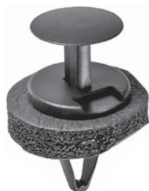
21672 (11611110) Black Nylon Cowl Vent Push-Type Retainer with Sealer Head Diameter: 18mm Stem Length: 20mm Fits into 6.3mm Hole Buick Allure & LaCrosse and Chevrolet Volt 2010 - On
