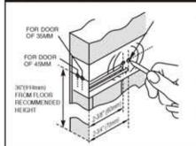
Place template on outside of door with height center line 36" from floor, Mark both holes as shown.
