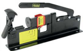
881540 Hose Cutter with Toggle This unique tool combines a hose cutter with a toggle action that presses the fitting into the hose, making every job easier, whether you are making one assembly or a hundred. It is designed to handle Push-Lok hose from 1/4" through 3/4".
