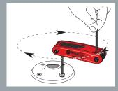
90° stop converts the tool into a non-stop, time saving, speed wrench.
