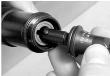
Locate mandrel pin in the slot of the driving spline and slide the front end assembly into the case.
