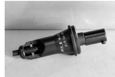
Finished front end assembly with mandrel wound through the pre-winder nozzle.
