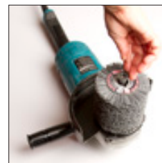
STEP 3. screw on the nut
