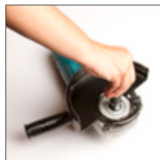
STEP 1. screw on the sleeve
