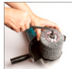
STEP 4. tighten nut with Allen wrench
