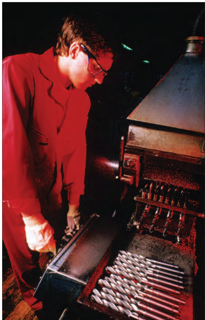
Flute milling of taper shank drills
