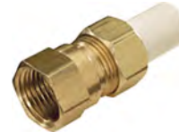
CPVC Female Threaded Transition Union (FIPT Brass x Spg CPVC)
