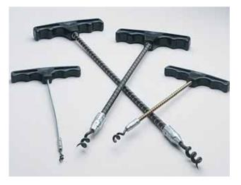
Chesterton 253 Flexible Packing Extractors are designed for strong pull packing removal. Construction features include high strength aircraft cable, precision heat-treated extracting worm, and unbreakable rotary-swaged assembly. Worm tips have plastic protective coating. Large, smooth, easy-grip handle. Furnished in sets of 4 tools. Set Reorder Number 002400
