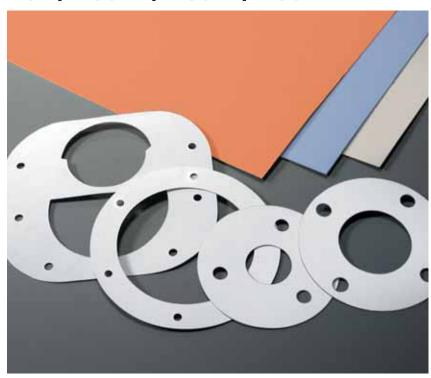
Chesterton **184** is 100% virgin PTFE with micro-fibrillated internal structure for excellent stability. Micro-fibrillated structure turns ordinary PTFE into a dimensionally strong, creep resistant gasketing material. 184 provides a long lasting, high reliability seal with minimum re-torque requirements. 184 is soft and pliable to conform to worn or uneven services and effects a tight seal. Cut your gaskets from a 184 sheet using just a pair of scissors or knife.
