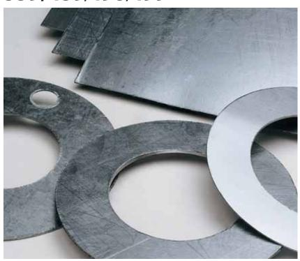
Chesterton **359** is a cost effective, general purpose graphite sheet reinforced with 304 Stainless Steel foil insert. Its excellent chemical resistance and thermal stability make this sheet a superior choice to compressed fiber sheet gasket for virtually all applications in the plant.
