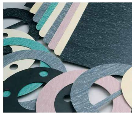
Chesterton **450** Synthetic Fiber Sheet is a low temperature, non-asbestos sheet gasketing material suitable for general services to 390°F (200°C). 365 psi (25 bar). 450 Synthetic Fiber Sheet is recommended for use in water, gas, brine and steam applications.
