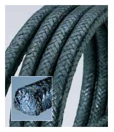
Chesterton 401 is constructed with wire-reinforced braided yarn which surrounds a flexible and resilient asbestos-free core. The non-asbestos jacketed yarn construction encapsulates the wire reinforcement in the yarn, preventing stem wear and scoring. This special construction makes 401 an economical, non-asbestos, general service valve stem packing for use in high-temperature and high-pressure applications.
