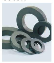
Chesterton's 5505H Flange Springs are specially designed, high-strength springs. They deliver a reserve of elastic energy to each bolt, allowing them to maintain constant load on the flange and gasket during normal operation, or during thermal cycles. Properly selected and installed, Chesterton's 5505H Flange Springs can provide dramatic improvements in leakage performance and service life.
