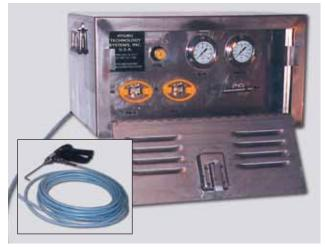
The Water Jet Packing Extractor system consists of an air operated, high pressure pumping system, high pressure hose, extraction gun, portable reservoir, and nozzle kit. This system has been designed for fast and efficient removal of valve stem packing, pump packing and flange gaskets. Reorder No. 104991
