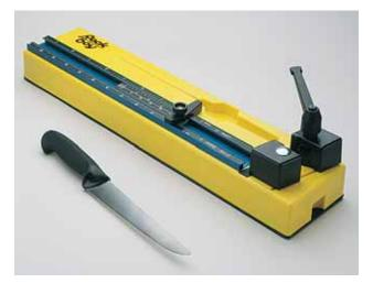
Chesterton 178 Ring Packing Cutter permits accurate cutting of rings from spiral or flat coil packings. The scale reads directly in terms of shaft sizes, in inches and in millimeters. To operate, simply set one scale to correspond with cross-sectional size of packing, set other scale for shaft diameter, and cut ring. Handles packing sizes 1/8" (3 mm) through 1" (25 mm) and shaft sizes up to 4" (100 mm). Reorder No. 003400
