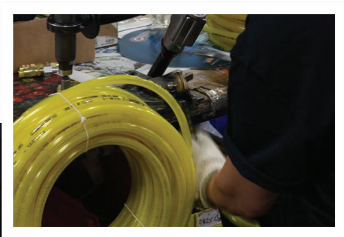
(Left) Installing fittings to Flexeel in our factory in New Jersey.
