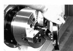
2. Adjust the forming devise to fit the bolt holes and turn the opposite direction of the chucks clamping force.
