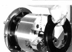
5. Unlock the chuck and remove the forming device.
