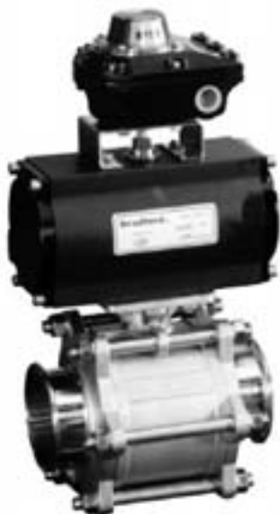
Bradford™ automated 3" encapsulated ball valve with direct mount double acting, (normally open), actuator and NEMA 7 (explosion proof with 2 mechanical switches) SPDT limit switch pictured. BV2CV-300CC-QAC.
