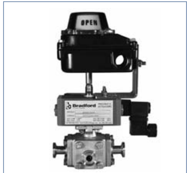
Bradford™ automated ½" 3-way 'L'-port encapsulated hygienic ball valve with double acting actuator and NEMA 4 limit switch with two SPDT mechanical switches and NEMA 4 115 VAC solenoid pictured. BV3SVLF050CBXC .
