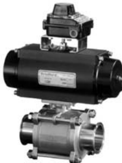
Bradford™ automated 2 1/2" 2-way encapsulated ball valve with spring return fail close actuator and NEMA 4/4X limit switch with two SPDT mechanical switches pictured. BV2CV-250CC-BFC.
