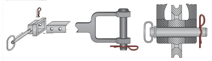
USED TO LOCK A HITCH PIN IN PLACE
