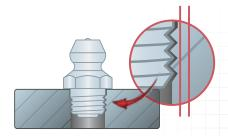
PARALLEL THREADS RUN PARALLEL TO MATING MATERIAL
