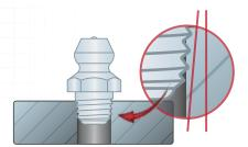
TAPER THREADS RUN DIAGONAL TO MATING MATERIAL
