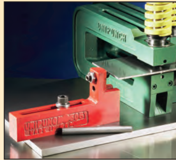
Typical 3-pin gauging Template Mounting
