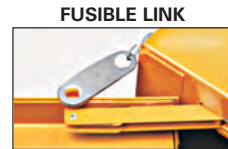
FUSIBLE LINK Fusible link holds doors wide open and melts at 165°F to automatically close (on self-close models).
