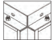
MOUNTING ANGLE FOR ROOMS WITH ROOF
