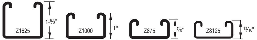
All Z-Strut is 1-5/8" Wide, With 7/8" opening
