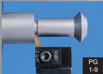
GROOVING AND TURNING .004" THROUGH .150" IN .001" INCREMENTS
