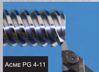
ACME EXTERNAL THREADING 4 THREADS PER INCH AND GREATER
