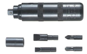
Klein Tools' Reversible Impact-Driver Set is a rugged, hand-impact driver designed to turn rusted, frozen, or other stubborn screws. The internal, spring-loaded, helical design transforms the impact of a hammer blow up to 200 ft.-lbs. of shock torque. It can also be used with 3/8-Inch square-drive impact sockets.
