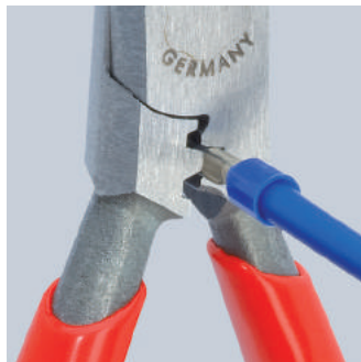
Crimping 20-14 AWG (0.5 to 2.5 mm 2 )
