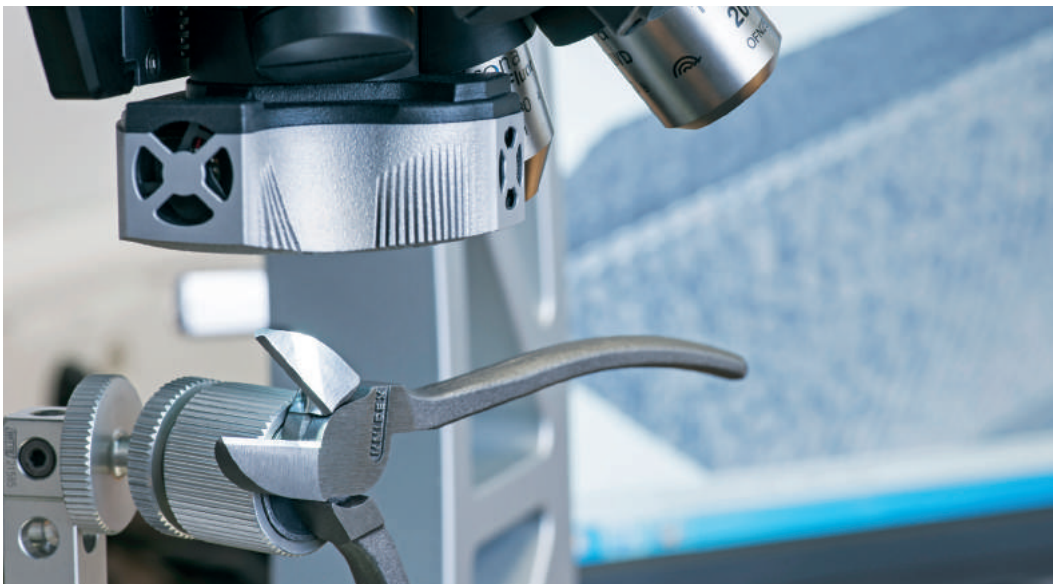
Shape and roughness of the diagonal cutter's cutting edge are precisely measured with an optical 3D measuring system.
