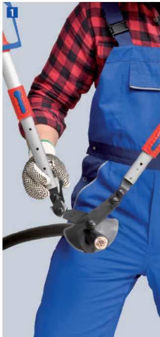
Setting of a favorable handle width
