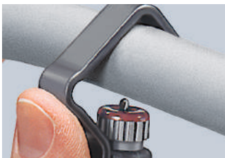
Setting the tool for circular cutting
