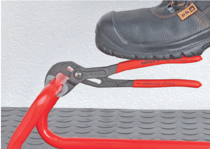
Teeth set against the direction of rotation have a self-clamping effect and prevent slipping off the workpiece
