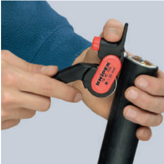
Setting the tool for longitudinal cut
