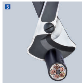
Thorough cut of the cable by repeat cutting and opening actions
