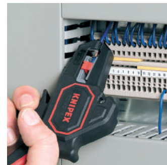
Stripping in confined areas
