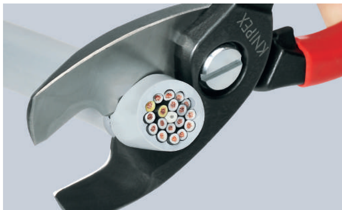
Final cut: after cutting the sheath in the front profile the conductors are cut in the rear area.
