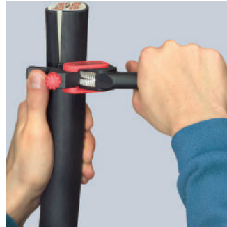
Turning the tool for circumferential cut
