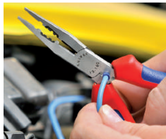
Crimping 20-14 AWG (0.5 to 2.5 mm 2 )
