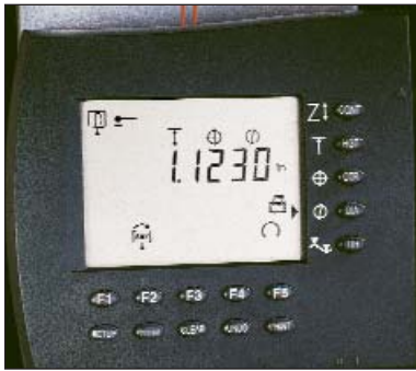
Large, easy-to-view / understand display shows the diameter of a hole or boss.
