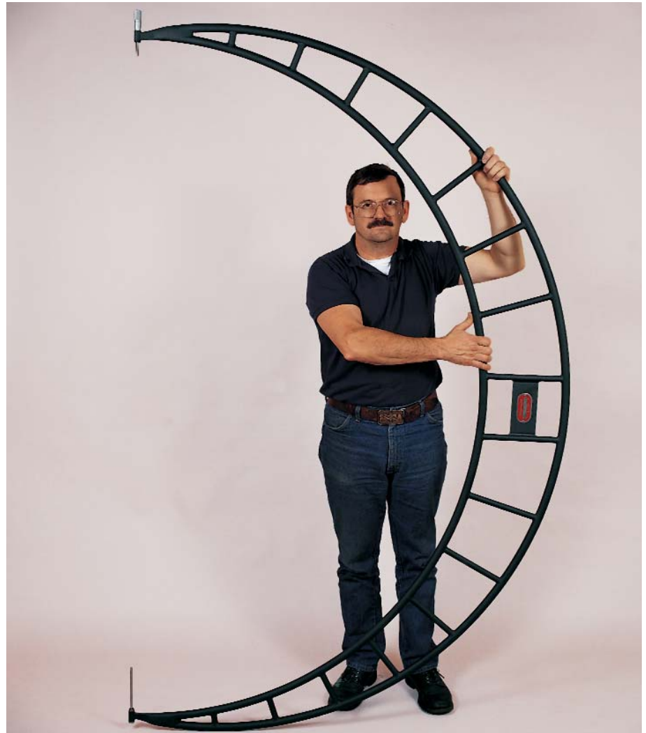
Starrett can manufacture extra large micrometers, like this special No. 724 Micrometer of tubing type construction, range 72-78" (1800-1950mm), with interchangeable anvils.
