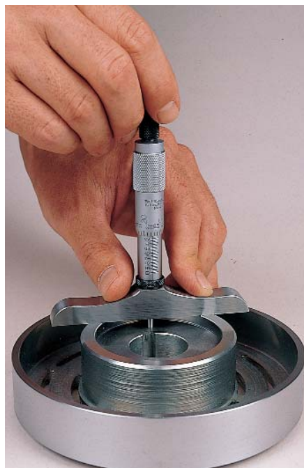
Measuring the depth of a shoulder with the No. 445AZ-3RL.
