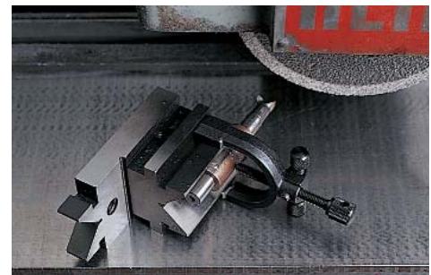
Sharpening cutter flutes.
