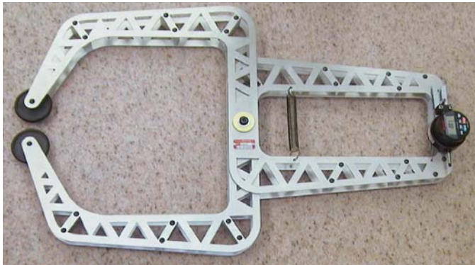
Large caliper with long reach for high temperature environment.
