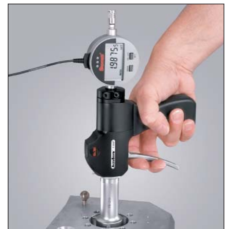
Output jack enables collection of measurement data for SPC analysis.
