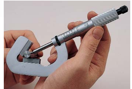
Checking out-of-roundness on centerless grinding work.
