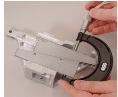
Top: Set No. S154LZ with No. 154E in foreground. Right: Checking inside measurement of slot with parallel and outside micrometer.
