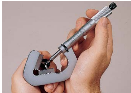
Measuring outside diameter of 3-fluted counterbore.
