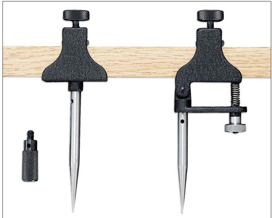
No. 50A Trammel Heads with points (adjustable point capability on right side head) mounted on beam (not furnished) for demonstration purposes. Pencil socket (lower left) can screw into a head in place of points if drawing (instead of scribing) is desired.
