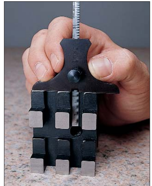
Right: Measuring depth of blind hole.
