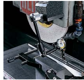
Left, No. 657A shown with No. 196B1 Universal Dial Indicator setting up workpiece on milling machine. Center, No. 657A with No. 711LS Last Word Dial Test Indicator setting up workpiece on surface grinder. Right, No. 657A.
