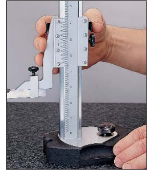
Quick-adjusting screw release allows rapid slide movement to desired area, then precisely positioned with the fine adjustment knob.
