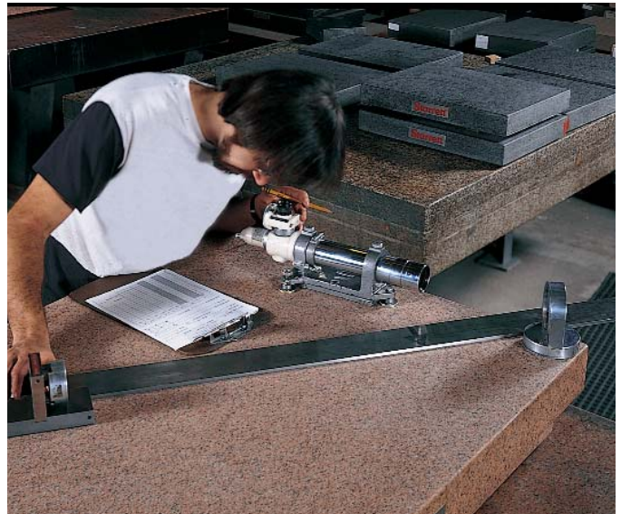
Inspecting a granite plate with an autocollimator.
