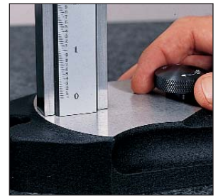
Precise positioning with fine-adjustment knob on the base isolates column and slide from external pressures.
