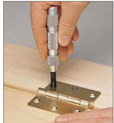
Automatically locates and centers countersunk holes and starting holes for screws, through hinges, latches, catches, etc.
