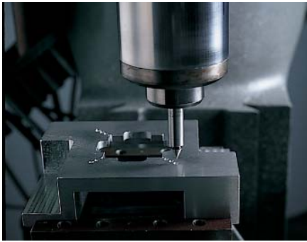
Locating the center with No. 827B.
