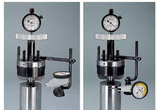
Below: Checking squareness (L) and external concentricity (R) using the No. 1141 Gage with Starrett No. 709 Test Indicator and attachments.
