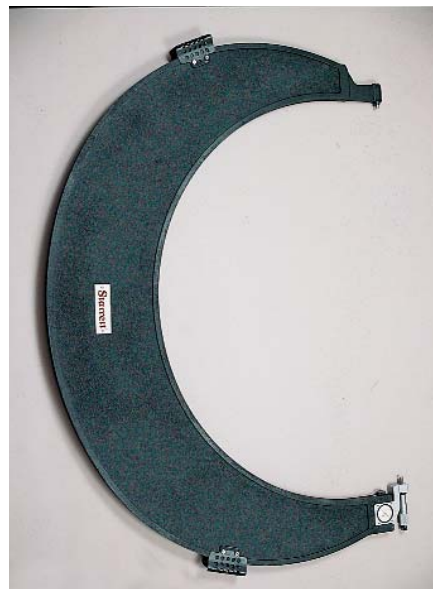
Starrett can manufacture extra large micrometers, like this special No. 724 Micrometer of tubing type construction, range 72-78" (1800-1950mm), with interchangeable anvils.
