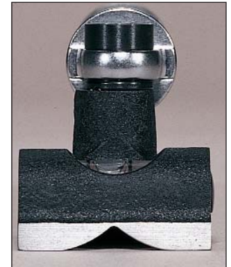
End view showing involute groove.
