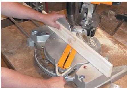
2. Set the saw to the angle that the Red Arrow points to on the Red Scale .
