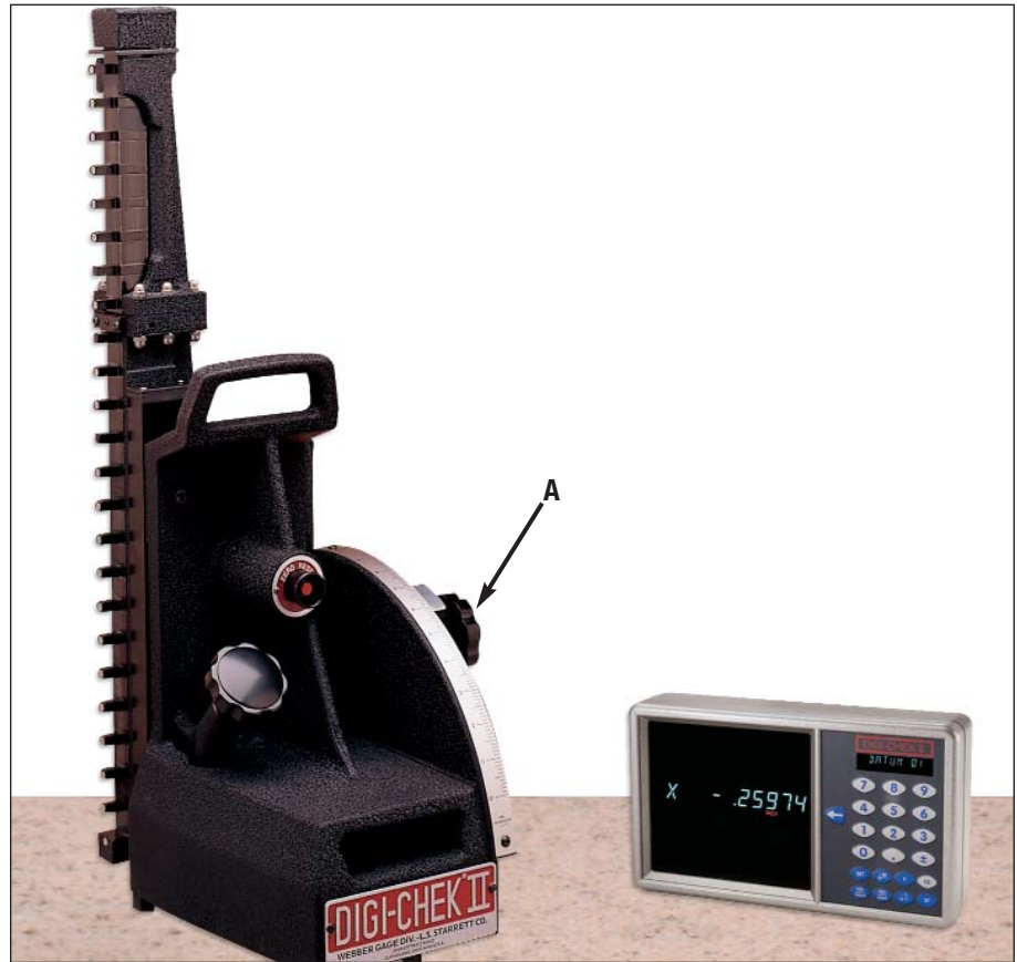
Simple, two step operation in less than 10 seconds. 1. Set rapid positioner (A) to within .005" (0.15mm) (3 seconds). 2. Final setting (5 seconds).
