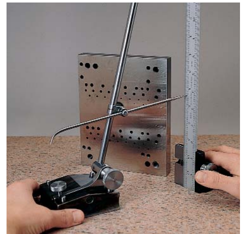
Transferring measurements with a Starrett Surface Gage used in conjunction with rule and rule holder.
