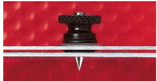
Side view of protractor with fulcrum point in place.
