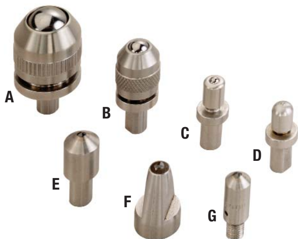
Penetrators: (A) 1/2" Ball Unit, (B) 1/4" Ball Unit, (C) 1/8" Ball Unit, (D) 1/16" Ball Unit and (E) Diamond Cone or "C" Regular. (F) Vickers/Knoop and (G) Newage-type indenter styles are also shown – contact Starrett for further information.
