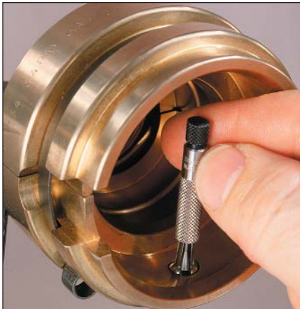
Measuring hole inside of coupling.
