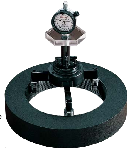
Below: Checking squareness (L) and external concentricity (R) using the No. 1141 Gage with Starrett No. 709 Test Indicator and attachments.
