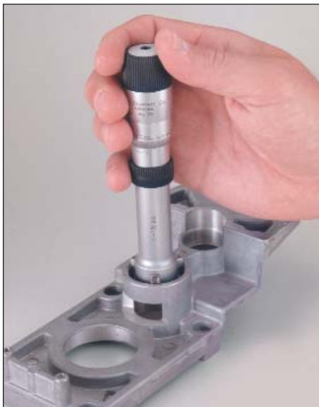
78XTZ-138 Measuring a bore.
