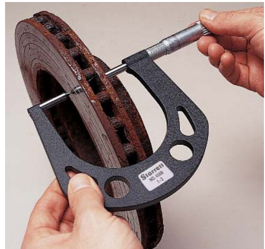
Measuring the wear groove depth on a disc brake with the No. 458BXR.
