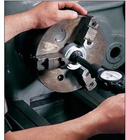
Above: Inspecting bore size with No. 84Z-111-4J.
