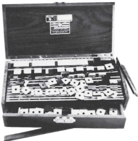
Example of a set damaged in transit due to improper packaging.
