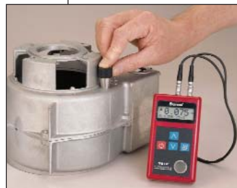
Measuring a wall thickness that would be difficult to gage with conventional hand tools.
