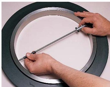
Measuring I.D. with micrometer and rod.
