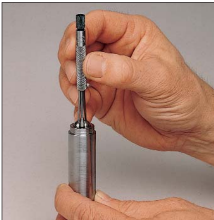
Measuring a small hole.
