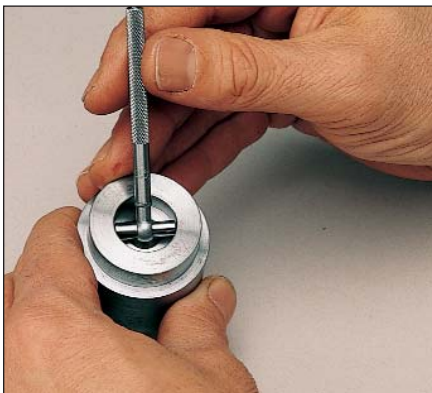
Checking a small hole.
