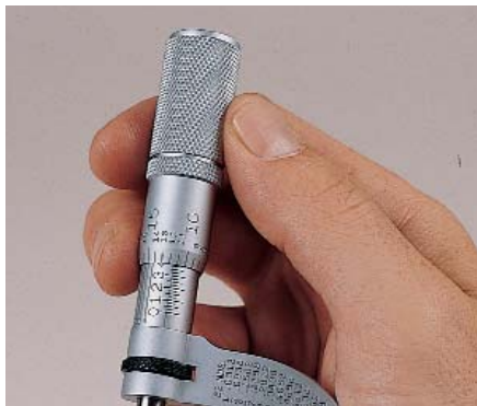
Friction thimble , smooth uniform pressure independent of “feel.”
