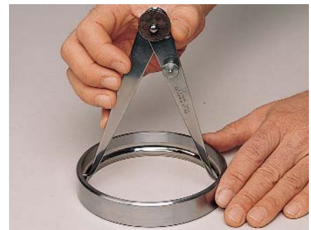
Checking inside groove.
