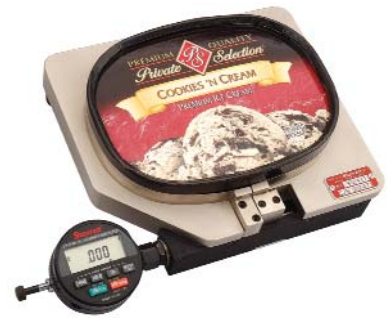
Top of 1-gallon container in measuring position.
