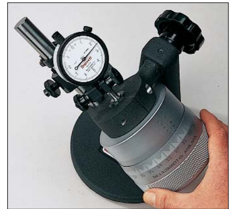
Checking AGD dial indicator.
