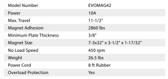
In the box: EVOMAG42, Keyed Chuck, Chuck Adaptor, Chuck Key, 3 Piece Handle, Safety Strap, 4 x hex keys, Safety Guard, Cooling Fluid Bottle & Tube, Carry Case & Instruction Manual
