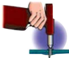
2 Using tool as a guide, insert rivet into prepared hole.
