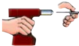
1 Insert rivet mandrel in rivet setting tool.
