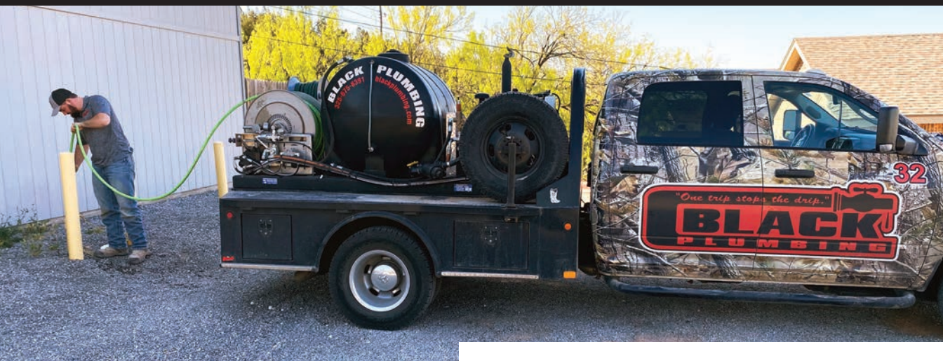
▲ Black Plumbing technician Layne Constance uses the PipeHunter trailer jetter mounted on the back of one of the company's service vehicles. The company also wraps his vehicles in camouflage to differentiate from competitors. (Photograph courtesy Black Plumbing)
