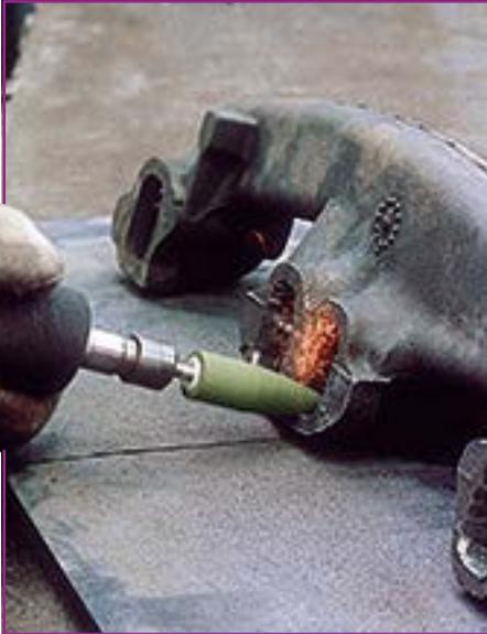
Resin bond, vitrified bond, center lap, and cotton fiber mounted points are available in a wide range of shapes.
