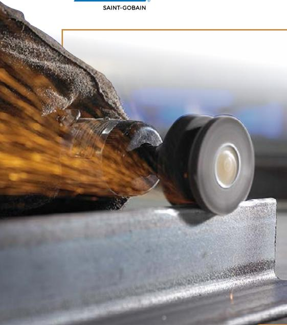
Flap wheels are an ideal choice for a wide variety of blending, deburring and finishing applications common in the metal fabrication and welding industries. Flap wheels are conformable to intricate shapes and contours. Designed to deliver a consistent finish with a uniform rate of cut, flap wheels wear away, continually exposing fresh abrasives.
