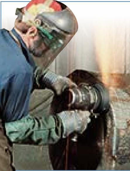
For consistent, quality performance in foundries, welding shops, fabrication facilities, steel mills and shipyards, Norton portable snagging wheels maximize your productivity. Used on horizontal/straight shaft grinders or right angle portable cup grinders.
