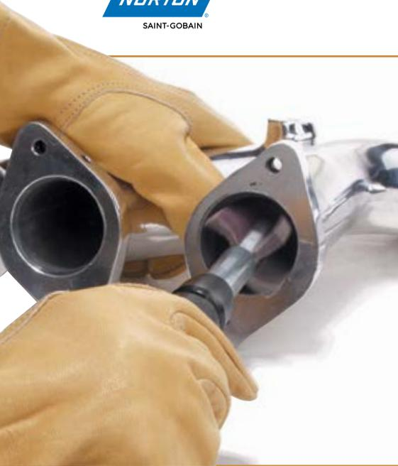
Flaps of abrasive cloth are stacked, inserted into a holder, and then attached to a mandrel. The flaps are designed to break down during use and reveal the next layer of abrasive.
