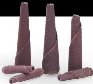
Good starting specification for flash removal, polishing, or removing machine tool marks and edge breaking on all types of metal in difficult-to-reach work areas
