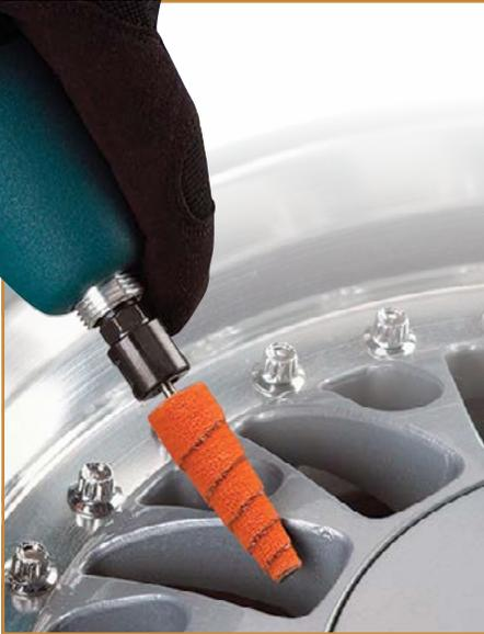
Spiral rolls are strips of abrasive cloth rolled and glued to form a solid shape that is designed to break down during use and reveal the next layer of abrasive.
