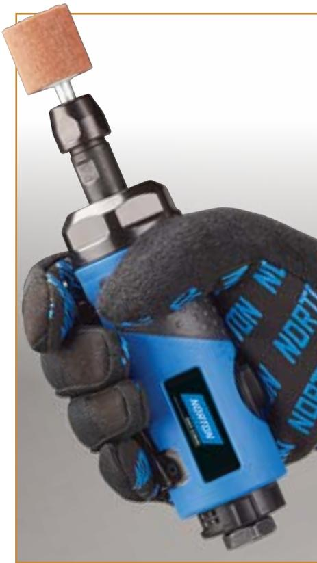
Our new Norton pneumatic die grinder quickly and comfortably accomplishes many portable applications without changing machines – including jobs for abrasive specialties (cartridge and spiral rolls...), small diameter flap wheels, mounted points, and carbide burrs.
