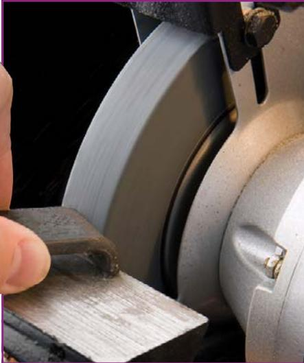
The Norton bench and pedestal wheel line consists of numerous wheel diameters and arbor sizes, abrasive types and grit sizes. Our offering answers all metal removal, deburring, shaping and sharpening needs: white aluminum oxide for high-speed tool steels, brown aluminum oxide for carbon steel, and silicon carbide for non-ferrous metals and carbide tooling.
