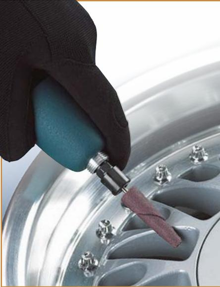
Tapered cone points are strips of abrasive cloth rolled and glued to form a solid shape that is designed to break down during use and reveal the next layer of abrasive. Tapered cone points are similar to cartridge rolls but their shape lends greater accessibility to many difficult-to-reach work areas. They are used for deburring holes and in close tolerance work areas.
