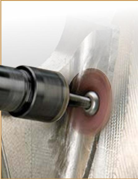
Square pads, cross pads and overlap slotted discs are all used on high-speed pneumatic tools for deburring, blending, cleaning, and polishing applications. All of these abrasive specialties are designed for applications in small, tight, hard-to-access locations on parts that are being finished.
