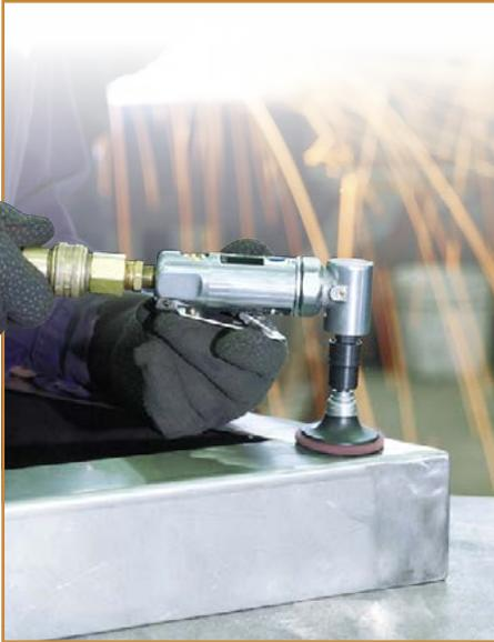
Non-woven quick-change discs are a combination of strong synthetic mesh and quality abrasives, bonded together by a smear-resistant adhesive. The open construction of the non-woven material enables aggressive cutting action and improved surface finish while maintaining its non-loading feature.
