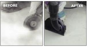
VACUUM REQUIREMENTS: QuikAttach™ will work with any vacuum, but for optimum efficiency use a vacuum rated at or above 11.5 amps (1.75 continuous hp) or 110 cfm.
