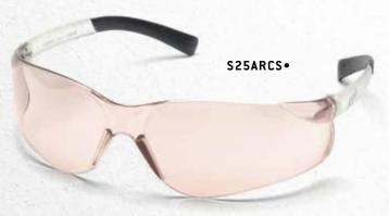
Designed for peripheral personnel and visitors who are NOT exposed to direct IR radiation. Great for use under the welding helmet - allows welder to see his work clearly without suffering "welders flash burn" from surrounding welders. Enhanced VLT (Visible light transmission) allows 58% of visible light to pass through the lens while blocking 75% of IR radiation. Doesn't distort color like green IR lenses.
