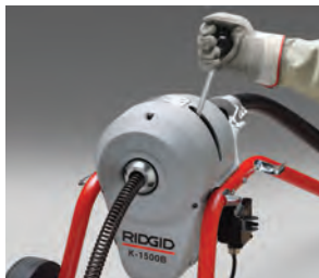
Release handle, cable stops instantly.
