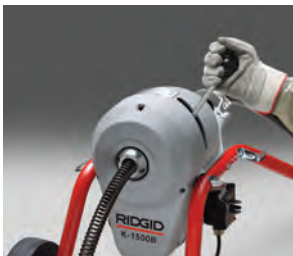
Engage clutch, cable spins.
