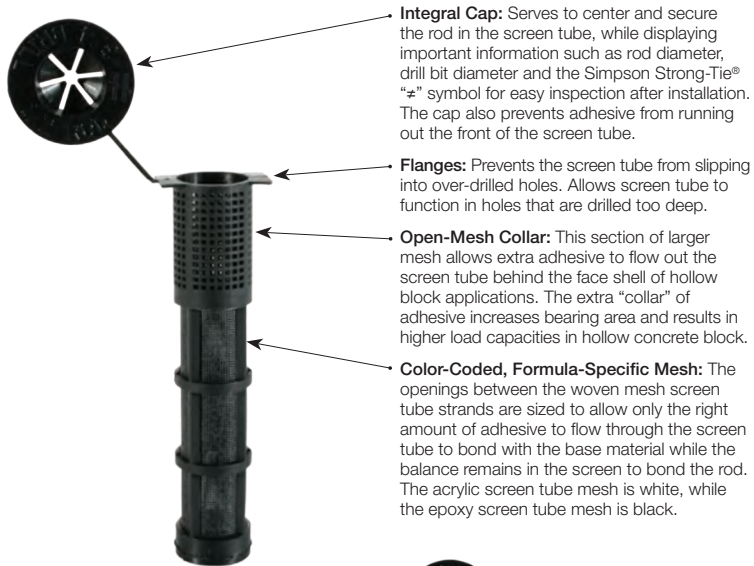
Epoxy Adhesive Screen Tube (mesh is black)
