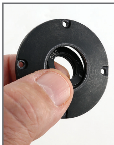
Insert Black Gold coolant ring into cap
