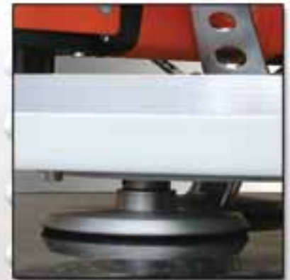
One of three 5" grinding platens (Velcro® surface)
