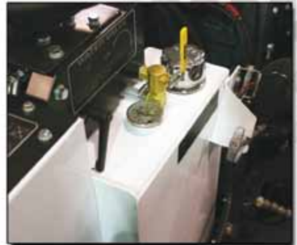
Upgraded, larger hydraulic oil tank
