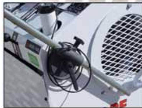
Adjustable pivot handles allow you to rotate the handle bars how you need them
