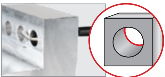
Hole Back-Edge For Sets: E, HC, U
