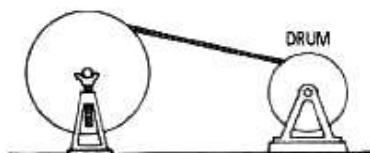
Fig. 4: A vertical unreeling stand. REEL (a) Correct REEL
