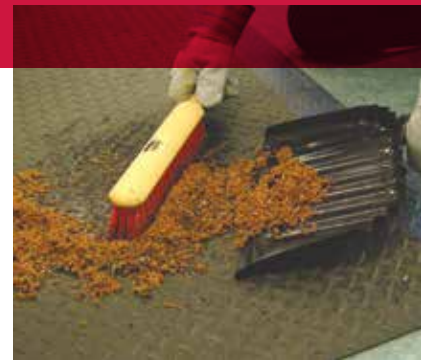
Cleaning up oil absorbent from a shop floor.
