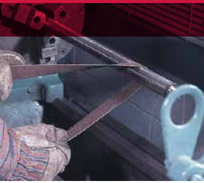
Polishing the O.D. of a part turning in a lathe.
