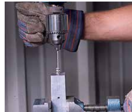
Crosshole deburring an aluminum manifold.
