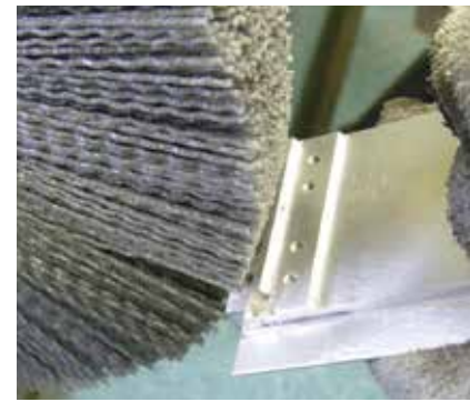
Removing burrs from an aluminum heat sink.
