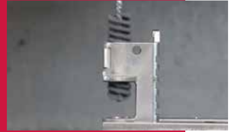
Deburring cross holes in a firearms component.
