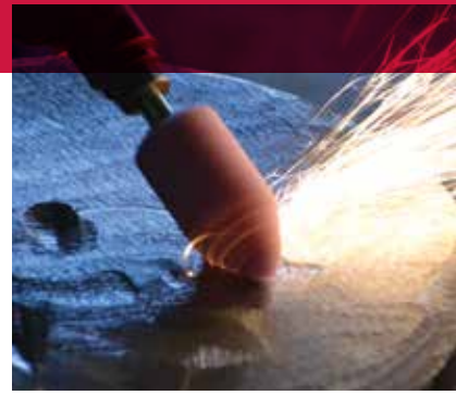
Tiger mounted points are ideal for light grinding in hard-to-reach areas and removing cracks from castings.
