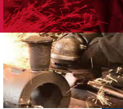
Riser removal with a type 27 grinding wheel.
