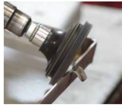
Edge chamfering a fabricated stainless component.
