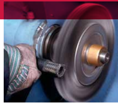
Removing rubber coating from a hydraulic hose.
