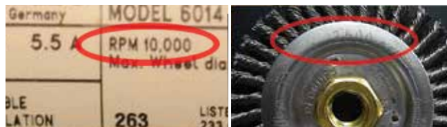
Match the RPM rating of the power brush to the tool being used. The RPM of the tool should never exceed the RPM of the power brush.
