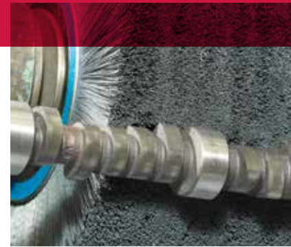
Deburring a camshaft with a Nylox wheel.
