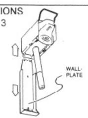
Separale dispenser from wall-plate by lifting upward on dispenser while holding wallplate.
