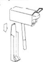
Mount dispenser on wallplate by first checking to see that aluminum cover is still pulled forward and then sliding the dispenser down onto the wall-plate.
