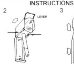
Be sure that screws are loosened. Press downward on the lever and then slide the cover forward.
