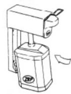
Mount a flat- shelf gallon bottle of Zep hand cleaner onto the dispenser by removing cap from the bottle and then sliding the bottle onto the intake pipe of the dispenser. The bottle should be pushed completely up to the top of the pipe so that the bottom of the bottle can be pushed inward to sit securely on the ledge at the bottom of the wall- plate.
