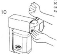
The dispenser is now ready to operate by pressing downward on the lever several times until the Zep hand cleaner is dispensed into the open hand.
