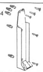
Mount wall-plate using wallplugs and screws supplied. (To mount on drywall please use appropriate fasteners. e.g. toggle bolts),
