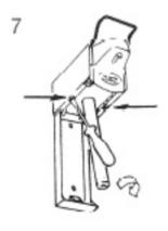
Tighten both screws on the bottom of aluminum cover.
