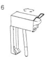
Leck dispenser onto wall plate by sliding aluminum cover tightly back into the slots on-wall-plate.
