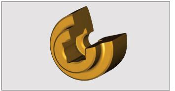
**Cornering Inserts** – Machine Squares, Hexagons, and Octagons with Inserts designed with two cutting edges intersecting at the appropriate angle 90, 120 or 135 degrees. Cut the corner, rotate the spindle (C axis) as required for the next cut (re-run of the subroutine) and repeat to completion. The same cornering Inserts may be used to generate a range of sizes of the given shape by simply increasing or decreasing the tool offset.
