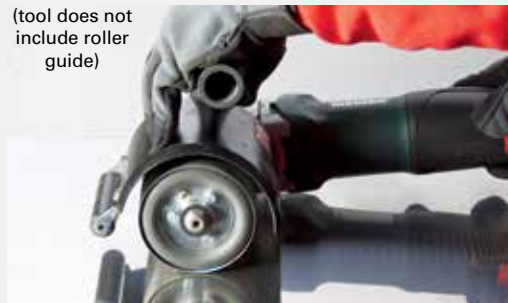
Preparation for mirror polishing: Metabo Burnishers with expansion roller, and Pyramid sanding belts from A160 (120 grit) to A6 (2000 grit).
