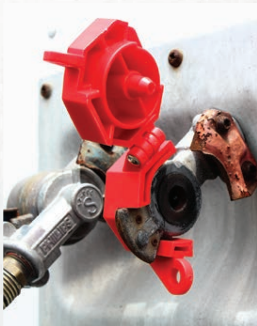
Attach device to Glad Valve.
