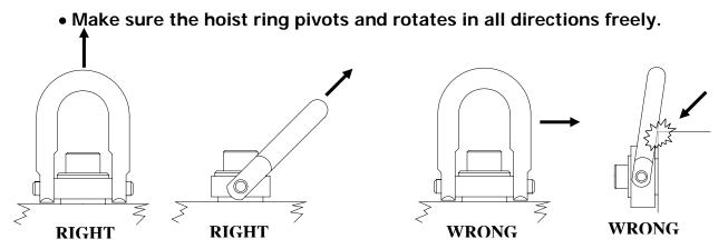
**Important**: The load on each hoist ring is not simply total weight divided by the number of hoist rings. The resultant force can be significantly greater at shallow lift angles and with unevenly distributed loads. See the example below.
