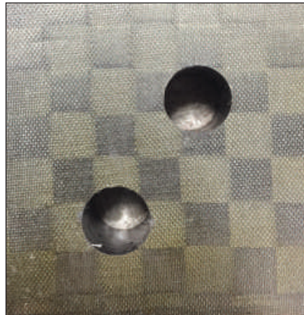
Holes drilled with PCD tooling
