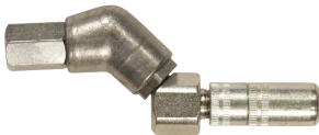
TIM-124* 360° Adjustable-Angle Standard Diameter Coupler Locks in place at 60° increments. Inlet thread 1/8" NPT (F). Overall length 3". 7,000 PSI maximum working pressure.
