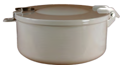
TIM-SPILL-BOX3 Lockable Spill Container Installed on above-ground tanks to contain small spills and drips from the fill nozzle. Removable screen allows for used filters to be drained. 2"(M) NPT riser connection. White powder-coated finish. 3-1/2 gallon capacity. ULC listed.
