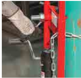
Chain clamping system secures cylinder for lifting and transport
