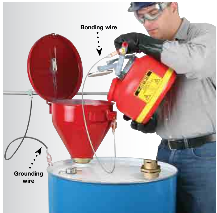
Proper bonding and grounding techniques prevent static discharge and the potential for fire.
