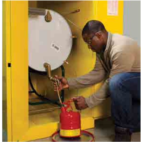
Use proper grounding techniques when dispensing flammable liquids
