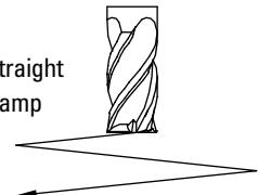
Alternative methods are helical and straight ramping. High ramp angles require reduced feed. Lower ramp angles will allow higher feed rates and extend tool life. Use slotting speeds and feeds for ramp angles of 1° to 2°. Reduce feed to 25% when ramp angles approach 6°. General purpose tools and/or difficult to machine materials will require lower ramp angles and reduced feed.
