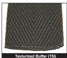
A bulked fiber is used to produce a thin webbing with good abrasion resistance.
