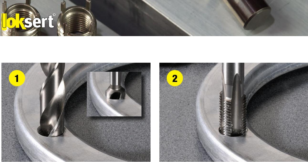
Drill with a standard tap drill and countersink with a standard 82°-100° countersink tool; see tables for correct dimensions.
