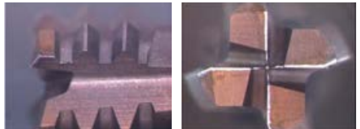
Epoch D Thread Mill after threading 600 holes.
