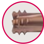
1 incomplete thread and 2 complete threads
