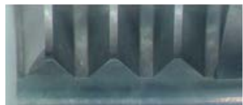
Epoch Thread Mill after threading 300 holes.
