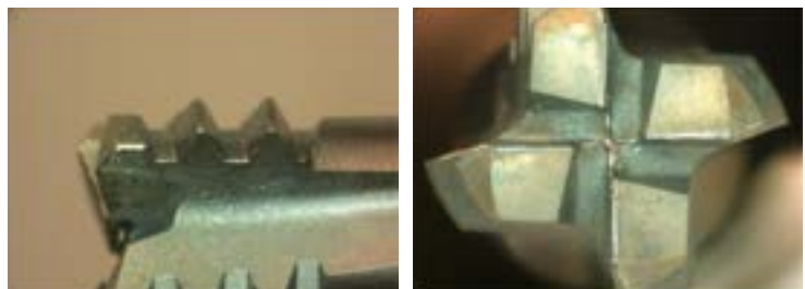
Epoch D Thread Mill after threading 150 holes.
