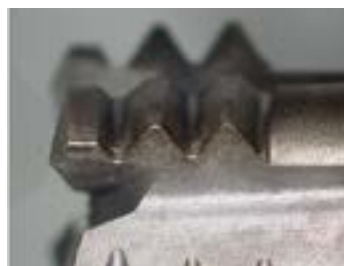
Epoch D Thread Mill after threading 50 holes.
