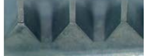
Epoch Thread Mill after threading 300 holes.
