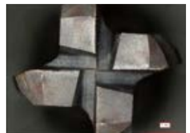
Epoch D Thread Mill after threading 50 holes.
