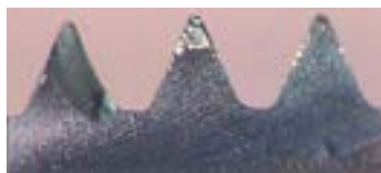
Conventional after threading 10 holes.
