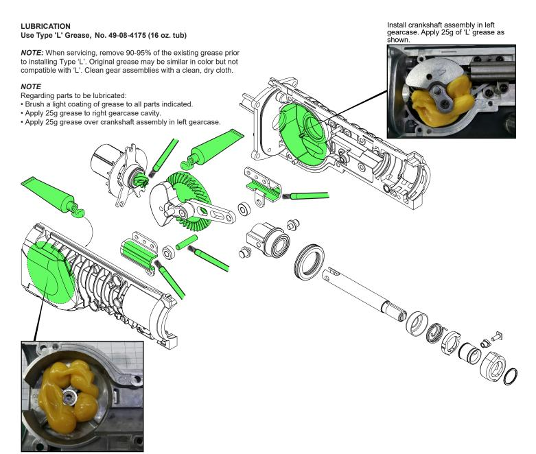
Place 25g of 'L' grease in right gearcase cavity.
