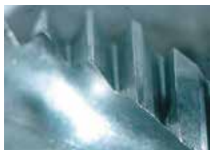
Cutting Edge after Tapping 1,000 Holes
