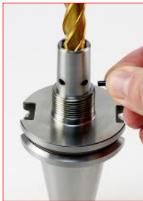
Insert the Hardened Dowel Pin
