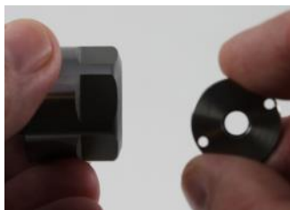
Thread Coolant Cap into ER nut, snug with wrench after the collet has been assembled.
