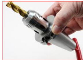
Adjust and Tighten the Preset Screw until tight against the Dowel Pin
