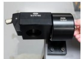
The tool holder will snap in automatically.
