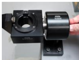
Push in on the Push Knob to unlock the head from the base
