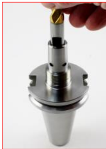
Insert the End mill, orientate the flat to the cross hole
