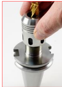
Assemble the Lock Nut Hand Tight
