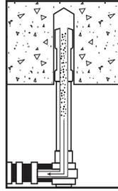
Drive the anchor into the hole until the anchor is at the required embedment depth.
