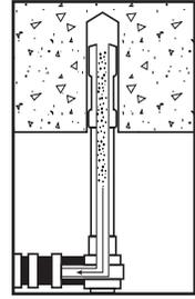
Drive the anchor into the hole until the head is firmly seated against the base material. Be sure the anchor is driven to the required embedment depth.
