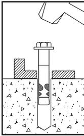
Drive the anchor through the fixture into the anchor hole until the nut and washer are firmly seated against the fixture. Be sure the anchor is driven to the required embedment depth.
