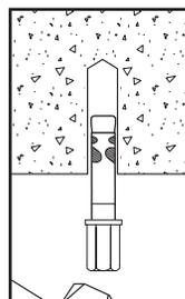
Tighten the coupler nut and washer up to the concrete surface and tighten the anchor by turning the nut 3 to 5 turns past finger tight or by applying the guide installation torque from the finger tight position.
