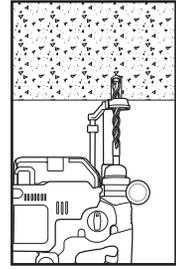
Remove dust and debris from the hole during drilling (e.g. dust extractor, hollow bit) or following drilling (e.g. suction, forced air) to extract loose particles created by drilling.
