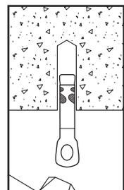
Tighten the tie wire nut by turning the head 3 to 5 turns past finger tight or by applying the guide installation torque from the finger tight position.
