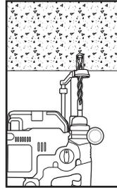
Remove dust and debris from the hole during drilling (e.g. dust extractor, hollow bit) or following drilling (e.g. suction, forced air) to extract loose particles created by drilling.
